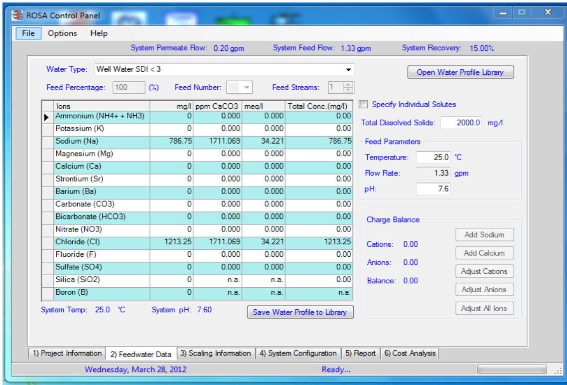
Figure 3-1. ROSA model feed water data interface.
